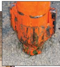
Upper photo, a close-up of the bottom of the cutter's pilot shaft, showing two opposing flanges. Below, a close-up of the teeth on the cutter.
