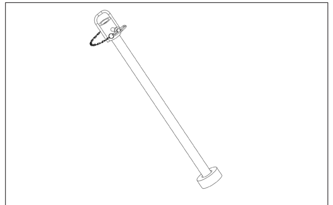
Figure 28. Newcon Plate Lift Shaft
